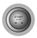
The keyless START/STOP Switch is located in the fascia to the right of the steering column, it is a push button style switch. To operate the switch the smart key must be inside the vehicle.
