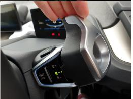
3) Release the parking brake by pressing the (P) button down with your foot on the footbrake. (the red light will turn off and you will feel the footbrake release slightly) Ease off the footbrake and the car will start to creep forward in D or backwards in R
