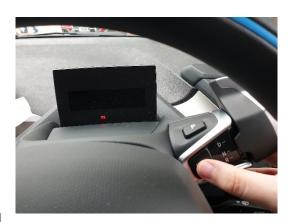
2) To select your gear, keep your foot on the brake and push the gear selector on the steering wheel away from you to move to D or towards you to N and R
