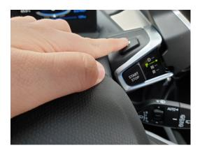
4) When parking the car press the Park button P on the gear selector whilst depressing the footbrake
